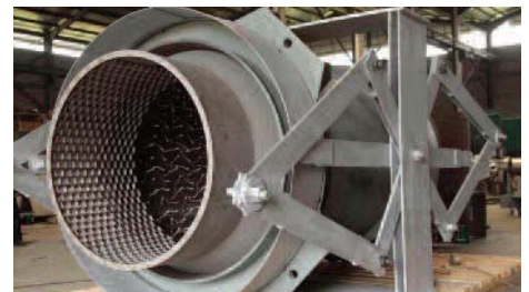
FCCU Expansion Joints
