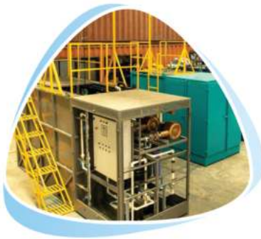
Electro Coagulation and Ozonation Treatment Systems
