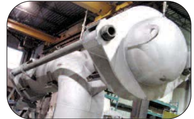
Elbow Pressure Balanced Expansion Joint
